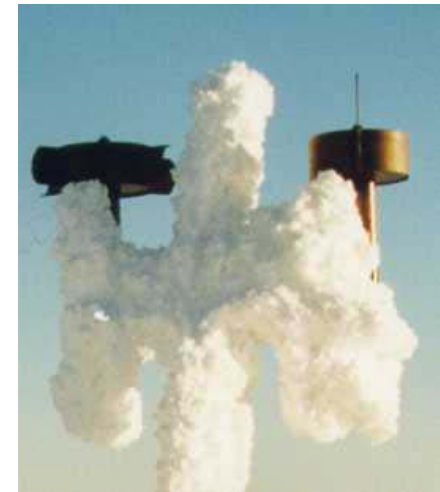
Rime ice on control anemometer and wind vane, Finland
